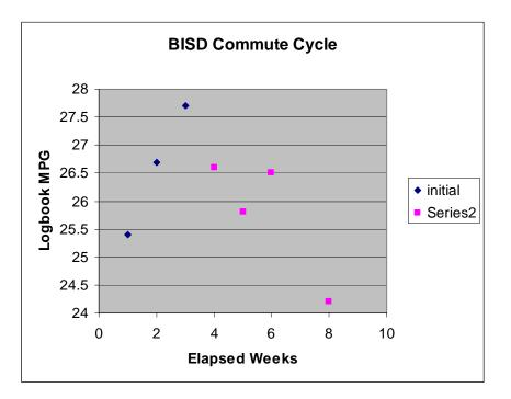
The driving cycle of the actual experimental gasoline baseline is the short-range (6 miles oneway) commute to MISD 5 days per week, with two complete round trips to MCC per week at 27 miles one-way. This 6 mile commute is shorter than the 10 mile warmup time, which tends to reduce fuel mileage further. The MCC trip is on a fully warmed car one way, but not the other. Ethanol performance is to be compared on this particular cycle. Data for the actual experimental gasoline baseline follow:
